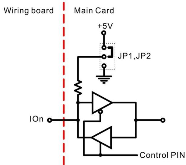
For byte-programmable TTL I/O IO00 ~ IO07, IO10 ~ IO17 to be configured as pull high or pull low. JP1,JP2 are used for output state of power on. (refer 7.3 JP1,JP2 Jumper setting)
