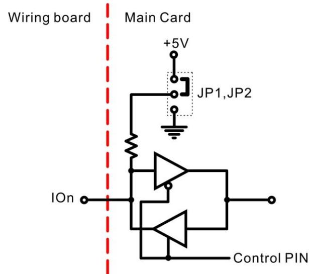
For byte-programmable TTL I/O IO00 ~ IO07, IO10 ~ IO17 to configured as pull high or pull low. JP1,JP2 are used for output state of power on. (refer 9.2 JP1,JP2 Jumper setting)
