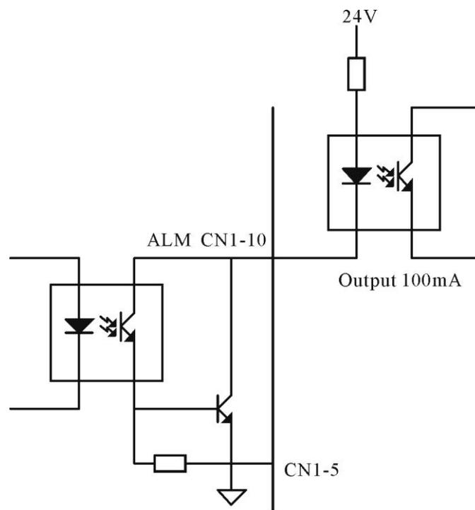
8.2 Encoder digital output interface circuit
