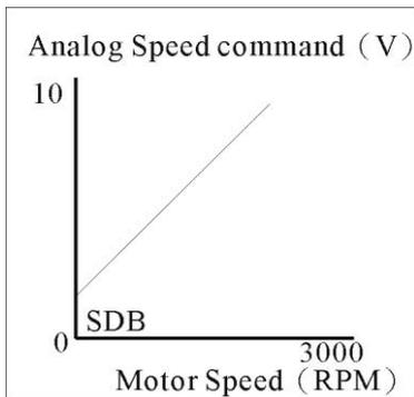
Minimum speed command can be set under the following situations:
