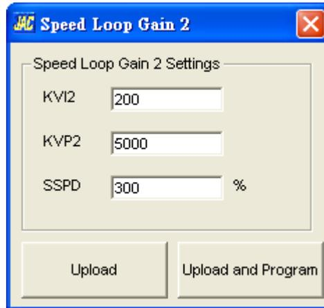
The KVI, KVP of speed loop gain2 is used as the speed is lower than SSPD setting value.
