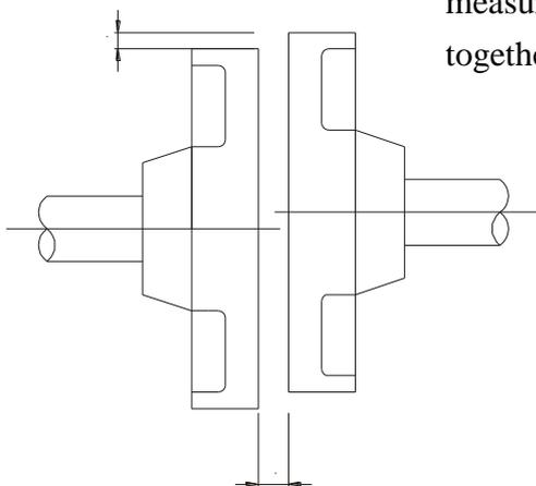
Measure this distance at four different positions around. The difference between the maximum and minimum measurements must be below 0.03mm (0.0012 in). (Turn together with the coupling.)
