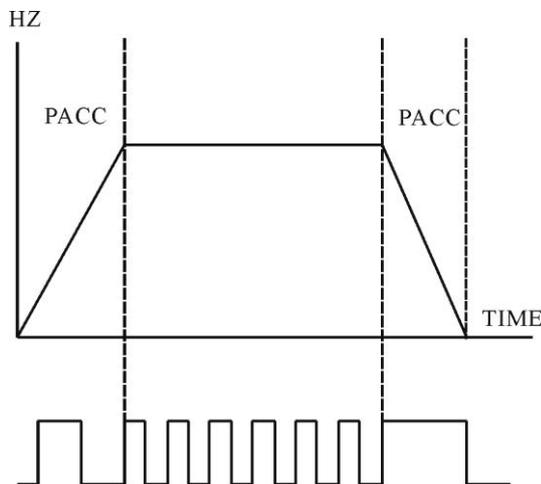
Under position operation mode this function can provide acceleration/deceleration function for the following situations:
