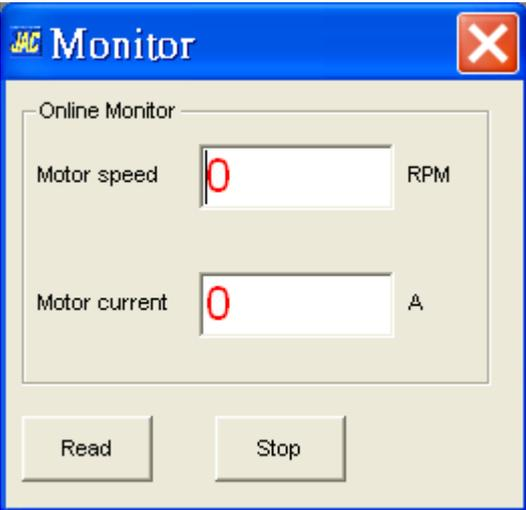
Use Read button to read the under monitoring data and stop to exit.
