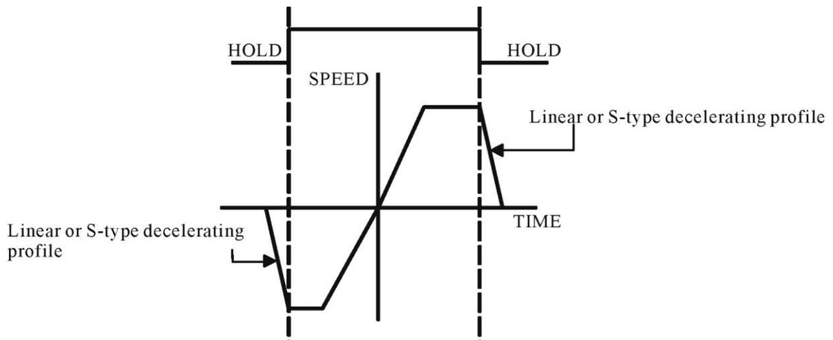
If PI/P Control Mode Switch function is selected, the speed loop will be changed from PI mode to P mode when CN1-16 is connected with 24G and. The mode switching function is described below:
