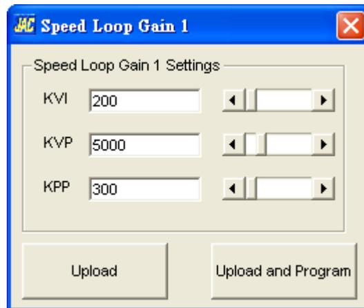
The KVI, KVP of speed loop gain 1 is used as the speed is higher than SSPD setting value.
