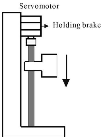
When the system power is turned off, the servomotor with brake prevents the movable parts from dropping due to gravity.
