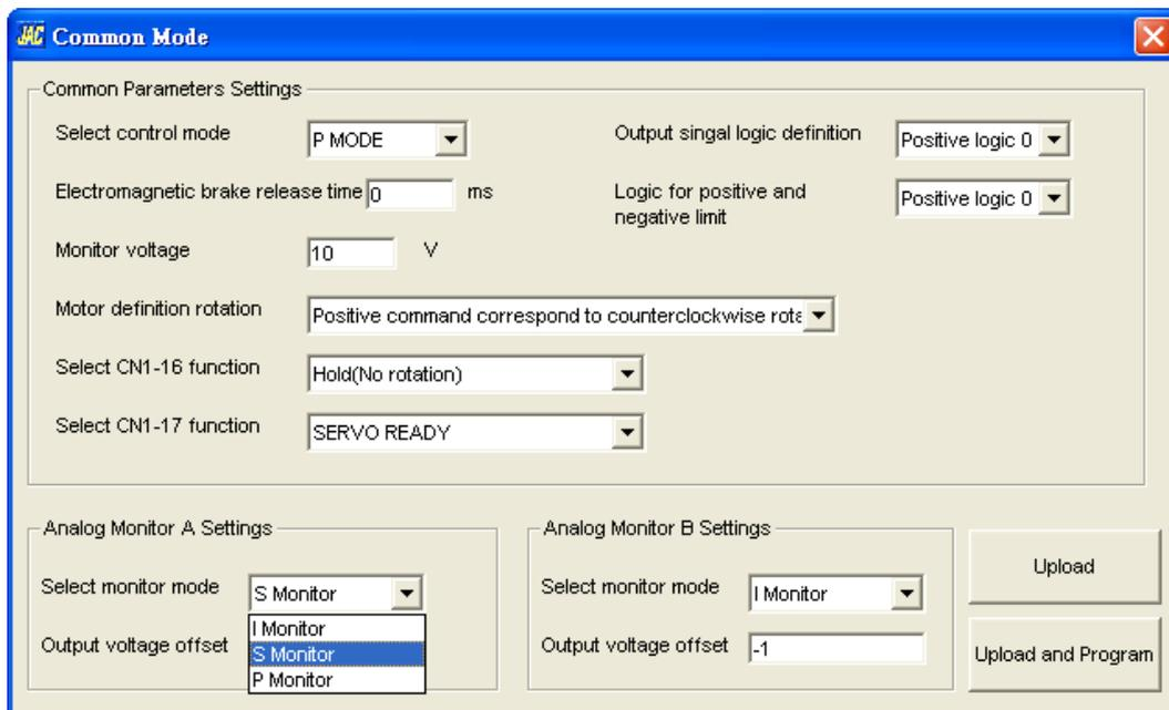
This field is used to set the maximum output voltage of the monitoring signals for both channel A and channel B, default value is 10V.
