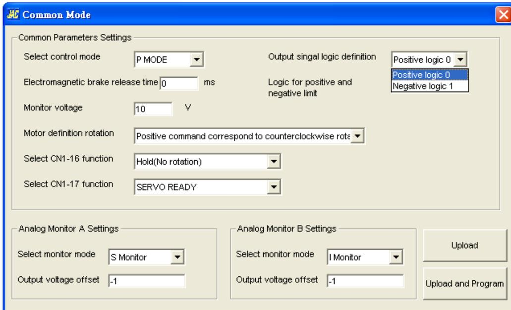
Define the logic of CN1-10, CN1-17, CN1-18, CN1-36, CN1-37 output signals
