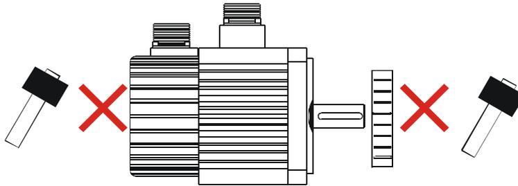
Avoid violent collision and vibration of servomotor when mounting a belt wheel or a clutch! The encoder connecting with the shaft is vulnerable under intense vibration which may adversely affect the resolution and service life of the servomotor.
