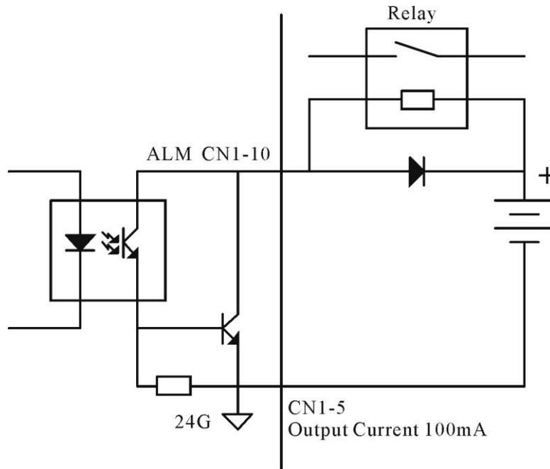
Example 2: Connecting to a photo coupler output circuit
