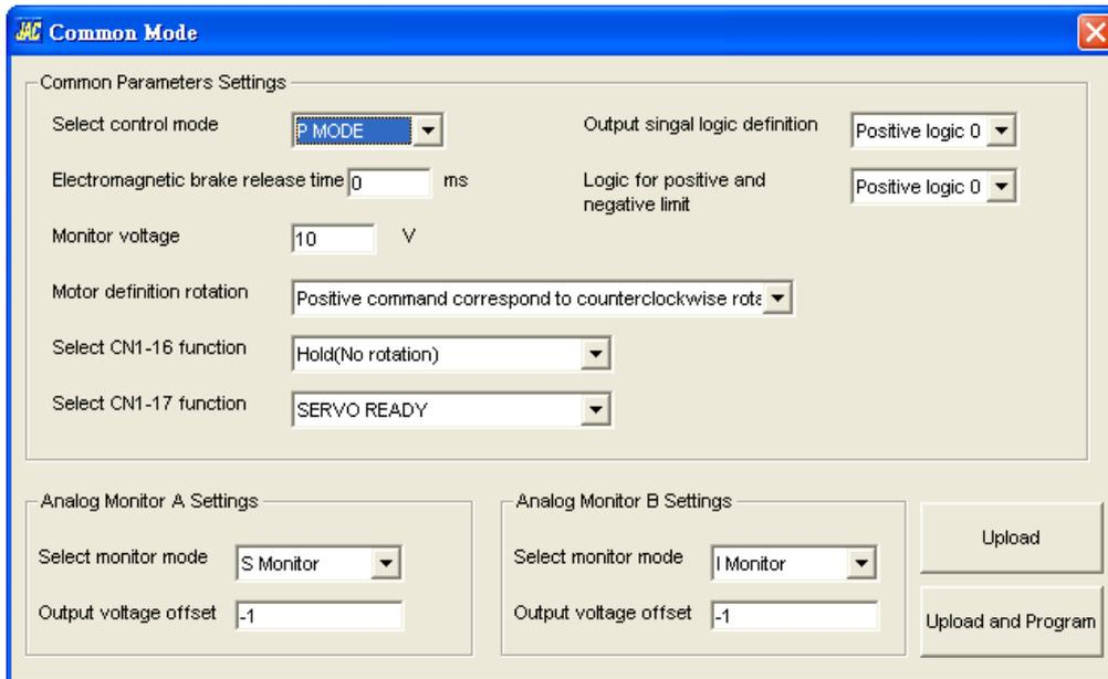
MBR is effective only when CN1-17 is programmed as the Motor Brake Release function.
