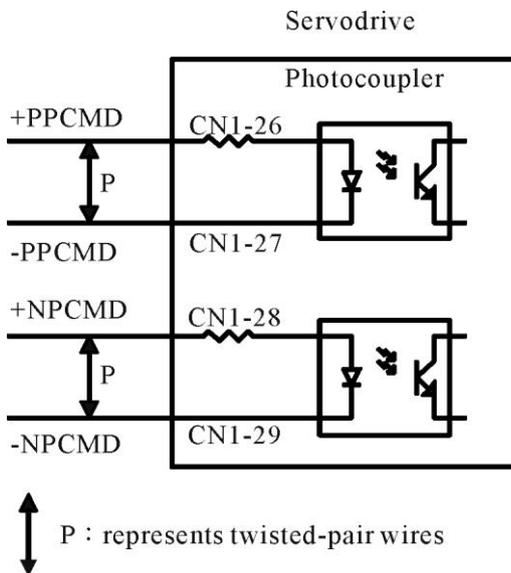
The position command signals can be any of the following forms (refer to 6. Position command input circuit):
