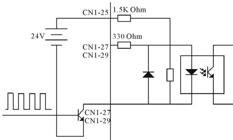
Example 2: Using power supply built in the servo drive
