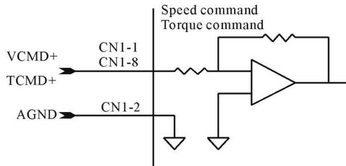
Note: CN1-1 is for high-resolution analog signal input (12 BIT). Please purchase YPV-XXX-V series servo drive if high-resolution analog input is needed. The input pin of the standard analog input (resolution 10 BIT) is CN1-8.
