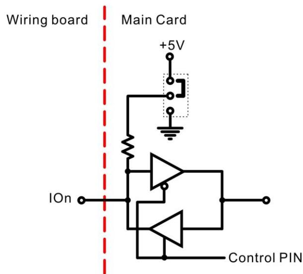
For byte-programmable TTL I/O IO0 ~ IO7 to configured as pull high or pull low. JP1 are used for output state of power on. (refer 8.3 JP1 Jumper setting)
