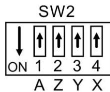
Example : A, Z axis are in negative polarity and Y, X axis polarity are positive, the DIP switch set as follows.
