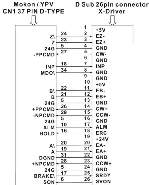
10.7 The wiring diagram for MPC3034A wiring board to Mokon / YJD servo driver
