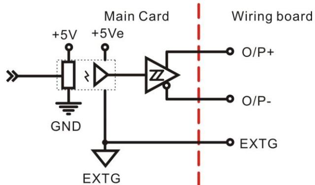
For motion control pulse output : CW,CCW
