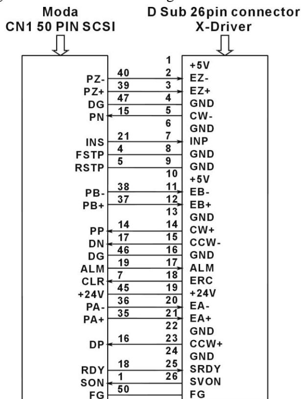
10.5 The wiring diagram for MPC3034A wiring board to YASKAWA servo driver
