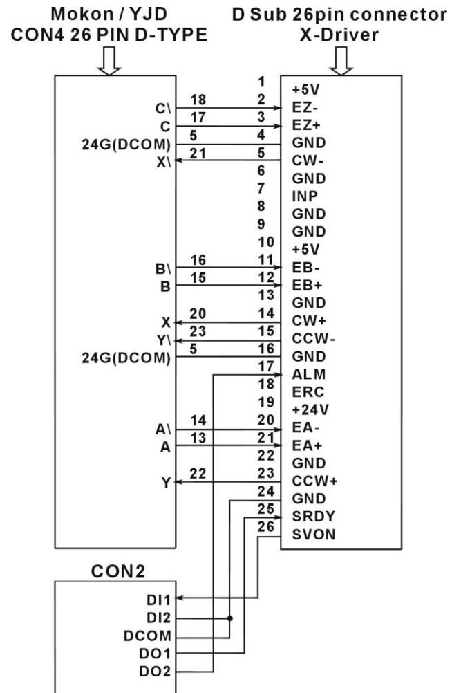
10.8 The wiring diagram for MPC3034A wiring board to MITSUBISHI J2-SUPER servo driver
