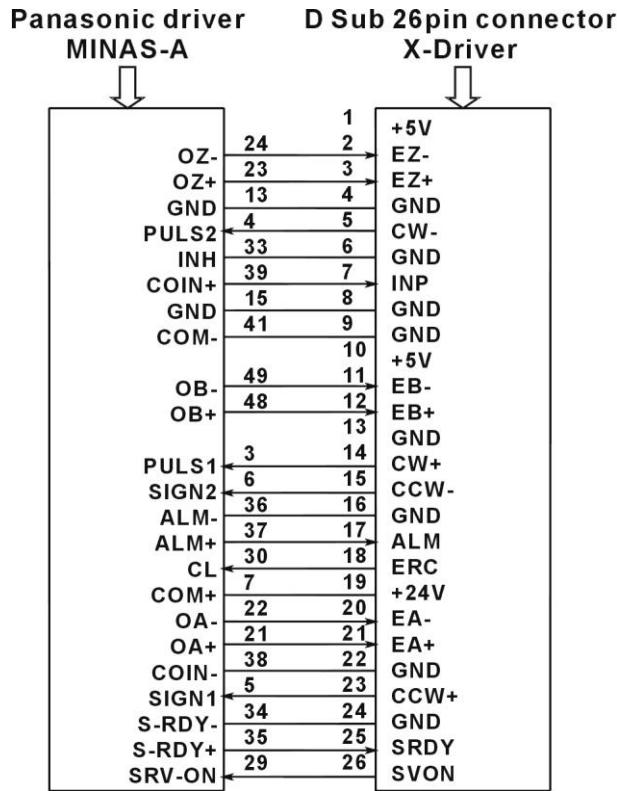
10.2 The wiring diagram for MPC3034A wiring board to panasonic MINAS MSD\*\*\* driver
