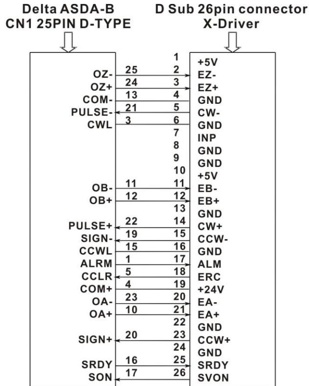
10.11 The wiring diagram for MPC3034A wiring board to Delta ASDA-B2 servo driver
