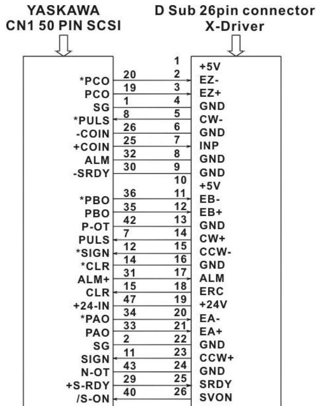
10.6 The wiring diagram for MPC3034A wiring board to Mokon / YPV servo driver
