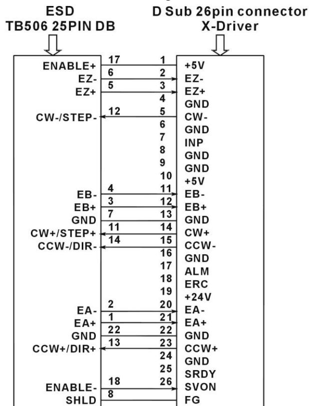
10.4 The wiring diagram for MPC3034A wiring board to Moda servo driver
