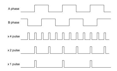
The left diagram shown that A phase leads B, if we take A leads B as up count and the counting pulse of up count will depends on the multiple rate.
