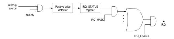
The interrupt source maybe digital input or timer/counter function. For digital input, the interrupt source is IN00~IN07, the physical input is changed polarity by
