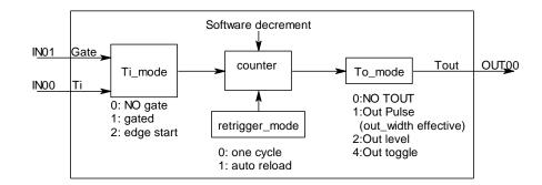
In this model, the counter can work in one cycle mode and auto reload mode.
