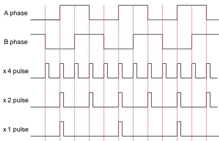
The left diagram shown that A phase leads B, if we take A leads B as up count and the counting pulse of up count will depends on the multiple rate.
