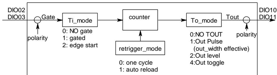
In this model, the timer can work in one cycle mode and auto reload mode.
