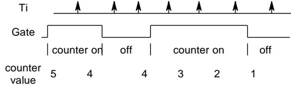
**Edge start:** the counter will start counting function while the gate input transition from inactive to active.
