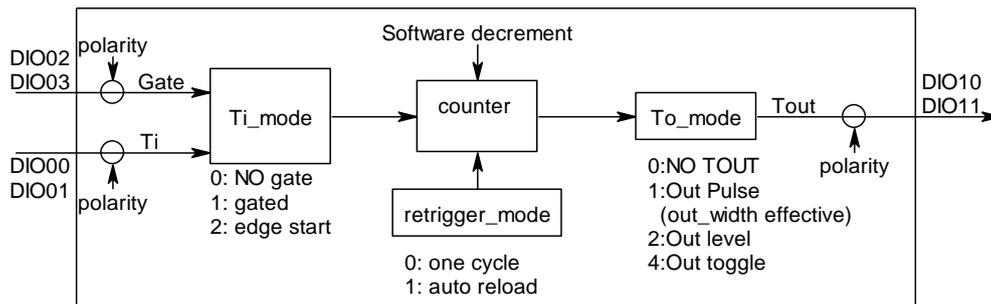
In this model, the counter can work in one cycle mode and auto reload mode.
