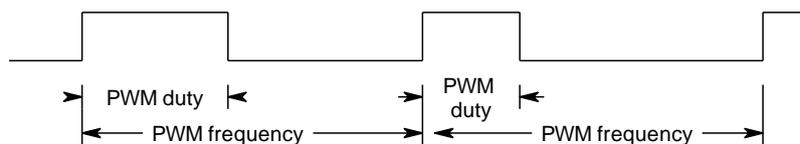
In this model, the PWM counter can only work in auto reload mode.
