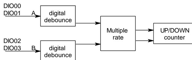
On the above diagram, you can see the digital debounce function filter out the unwanted high frequency then pass the signal to the multiple rate circuit to determine the pulse and direction, finally the counter counts the pulses.
