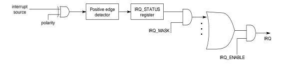
For digital input, the interrupt source is IN00~IN07, the physical input is changed polarity by POLARITY\_SET, then the on board hardware detect the positive edge transition to trigger the IRQ\_STATUS register, it is irrelevant to the IRQ\_MASK. If the IRQ\_MASK is set to 1 and IRQ\_ENABLE are also set, the interrupt will generate. By this model, you can see that you can check the fast changing input by IRQ\_STATUS without using interrupt.
