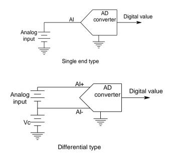
From the above diagram, you can see the differential type must have a common connection between measured signal and the AD converter. The under measure voltage is riding on a common voltage Vc.
