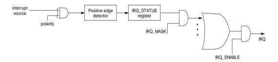
For digital input, the interrupt source is IN00~IN07, the physical input is changed polarity by POLARITY\_SET, then the on board hardware detect the positive edge transition to trigger the IRQ\_STATUS register, it is irrelevant to the IRQ\_MASK. If the IRQ\_MASK is set to 1 and IRQ\_ENABLE are also set, the interrupt will generate. By this model, you can see that you can check the fast changing input by IRQ\_STATUS without using interrupt.
