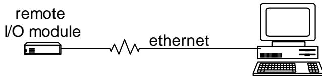
The module response or be commanded by the controller through Ethernet by UDP protocol. As a member on the Ethernet, it must have a distinguished IP and a predefined port. At factory, we set the default IP at 192.168.0.100 and the port at 6936 for the remote module.
